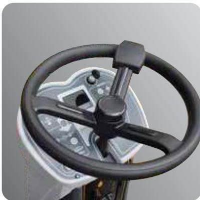
New control panel with digital controls and display. Digital display: with hour meter, battery charge level indicator, empty water tank level indicator, forward/reverse traction indicator. Speed control adjustment, horn, suction motor switch with delayed switch-off, brush plate lifting/ lowering selector switch, brush motor switch.
