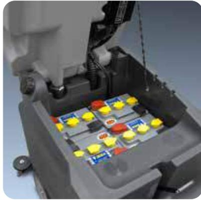
Great working autonomy thanks to the possibility to use 4 batteries 6 V 180 Ah granting continuous working up. Possibility to use also 2 batteries 12V. Less battery consumption thanks to rear wheel-drive. Large load tanks made of shock and acid proof polyethylene (real load of 85 l.), avoiding frequent stop for refilling.
