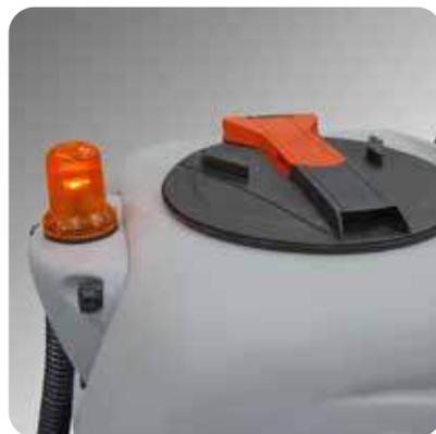
Quick lock recovery tank cap allows for fast and easy cleaning and sanitification of the tank; the tilting tank together with a large size drain hose allow the complete emptying of the tank and the removal of any type of solid dirt. The antifoam device protects suction motor, as well as the electronic floating switch that stops suction when the tank is full.
