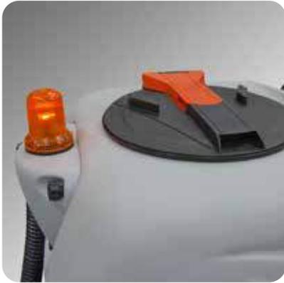
Quick lock recovery tank cap allows for fast and easy cleaning and sanitization of the tank; the tilting tank together with a large size drain hose allow the complete emptying of the tank and the removal of any type of solid dirt. The antifoam device protects suction motor, as well as the electronic floating switch that stops suction when the tank is full.
