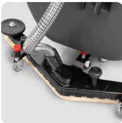
Renovated squeegee with new pressure adjusting system. The squeegee blades are easily replaceable without the use of tools. Quick and easy squeegee coupling through the two large knobs; the squeegee is released without any damage in the event of accidental impact.
