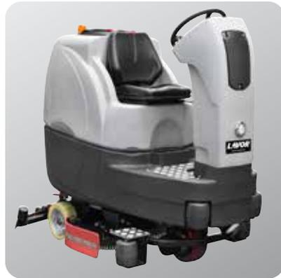
New brush plate 1000 mm for increased working capacity. Implementation of the ECO MODE function for brushes and suction to reduce energy consumption and noise. Acquastop kit to allow solution tank refilling without the operator's presence. Automatic brush attachment and release. Possibility to use Li-Ion batteries. The distribution pump of the solution allows an optimal solution distribution in relation to the speed.
