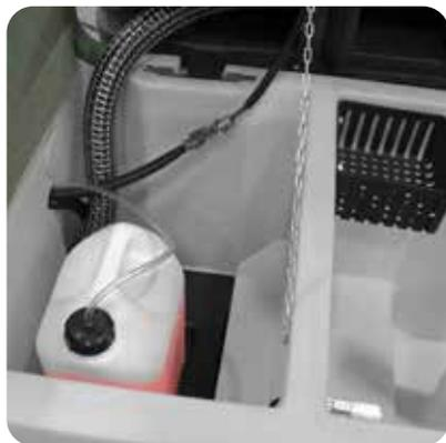
Automatic detergent dosing system (only for model code: 8.525.1301 - 8.525.1302)
