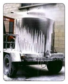
Continuous pneumatic foam sprayers need a permanent connection to an air compressor; in this way air mixes with the chemical product producing a soft and voluminous foam that persists on surfaces: with a little chemical product, it is possible to treat wider areas or tough dirt (also on ceilings, inclined and/or slippery walls). They work at high-pressure and so they use capacious steel or stainless steel tanks to allow a greater working autonomy.
