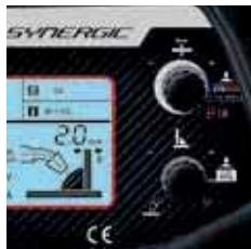
Set the material thickness and start welding!
